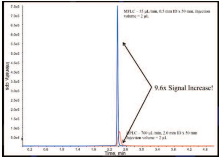
Figure 1. LC-MS/MS Overlaid Chromatograms (HPLC vs. MFLC) from Bioanalysis of Methotrexate (400 ng/mL) from Human Plasma Using Eksigent ekspert microLC 200 and a QTRAP 5500
