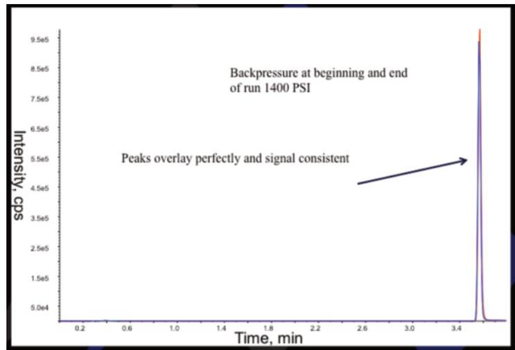
Figure 2. MFLC-MS/MS Chromatograms Overlaid from Beginning and End of Run of >350 injections of MTX Extracted from Human Plasma
